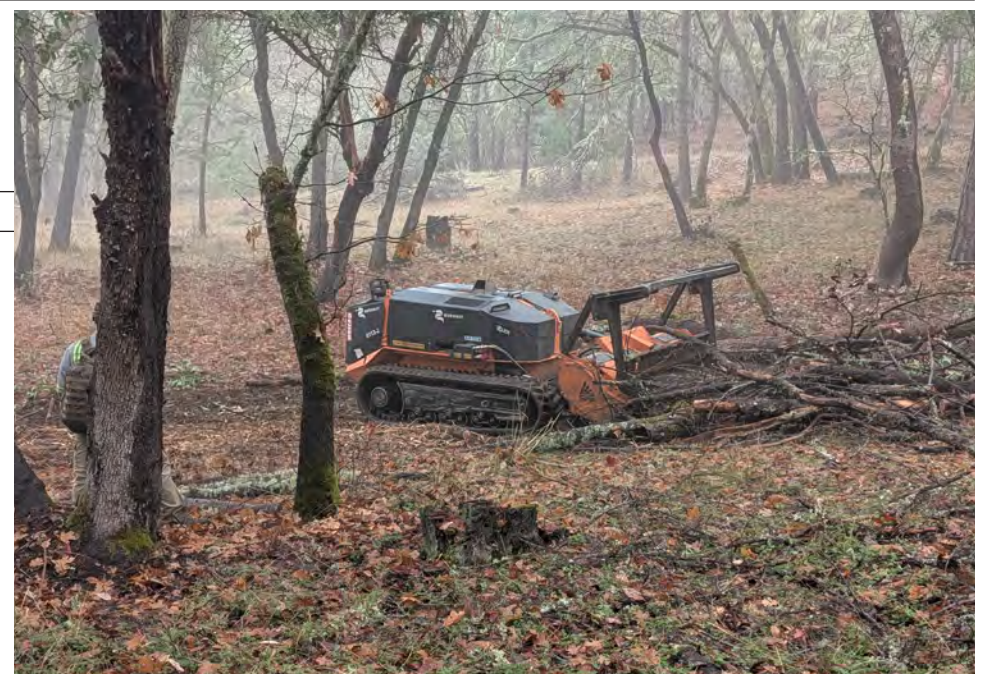
Pictured is a FAE RCU 75 rubber-tracked, remote-controlled masticator used by BurnBot on Applegate Partnership & Watershed Council (APWC) fuels reduction projects in the Upper Applegate. Photo by Nathan Gehres, APWC.
